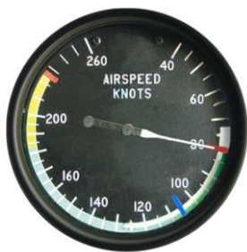
Figure 36. Air speed indicator Part 23 airplane with red V MCA and blue V YSE radial lines.
